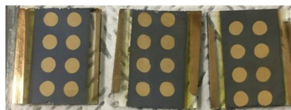
Figure 3. Growth CdS/CdTe/CdCl 2 /Cu/Au thin films in the AMRel.
